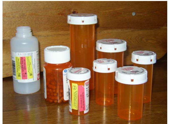
Examples of prescription containers. All amber vials are PP. The unpigmented container is not marked with a resin identification symbol (above).
