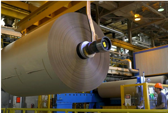
The B25 machine, which produces recycled corrugated medium and linerboard for packaging, at the Biron, Wis. mill. | Courtesy of ND Paper
