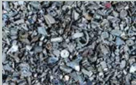
*Consistent, high quality sorting output (clockwise from top left): aluminum; copper; grey metal; brass. Grain size of material can be 10 mm or more with sorting widths of 1, 2, or 3 meters (x-ray version available in 1 and 2 meter widths only).*
