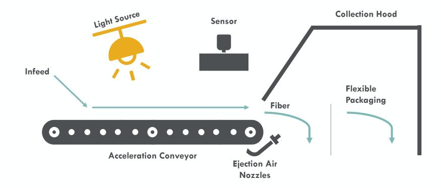
Successfully sort flexible packaging from paper through addition of optical sorters on fiber lines, airflow controls, collection hoods and other system adjustments.
